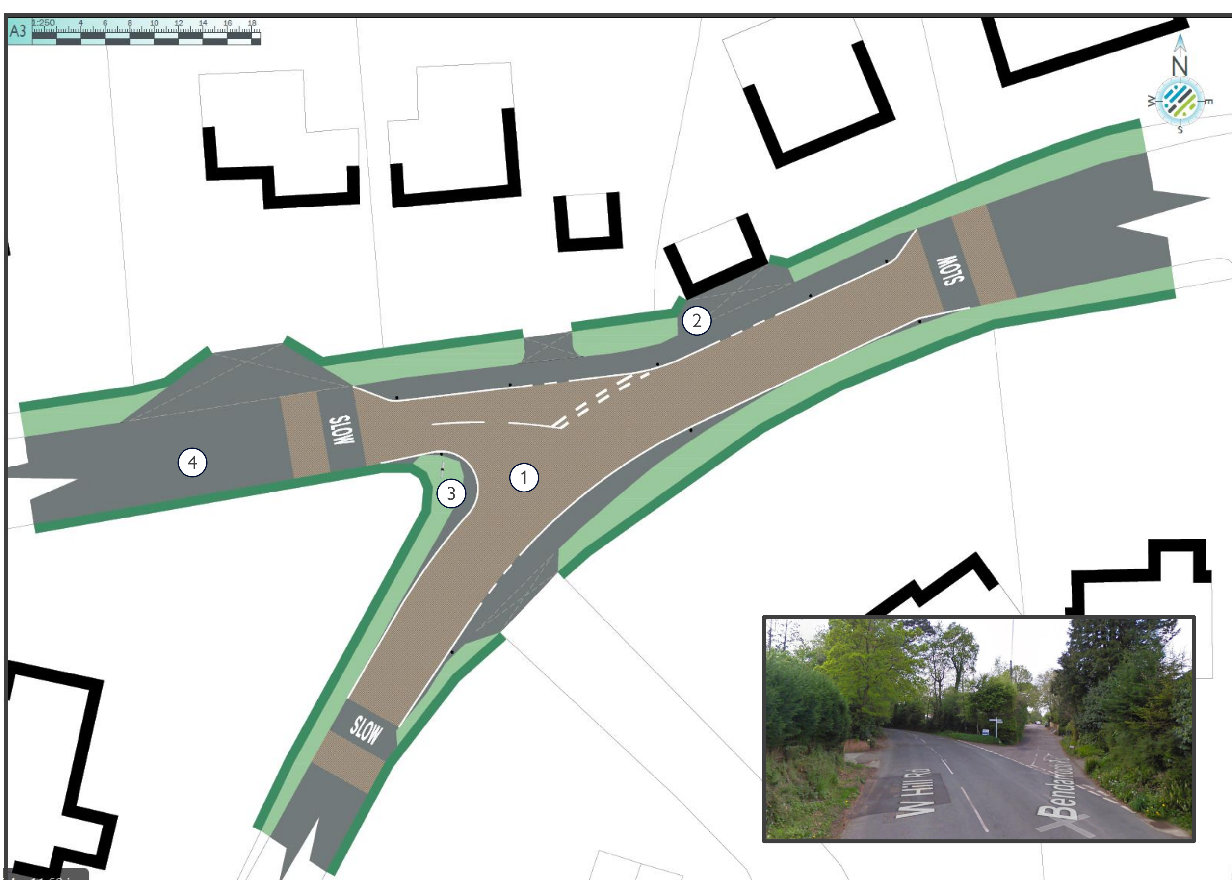
Feasibility design showing junction of Bendarroch Road / West Hill Road
